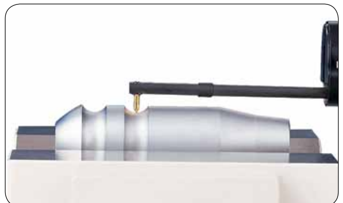
Measure dimension, form and texture at once with a single traverse over curved or straight surfaces
