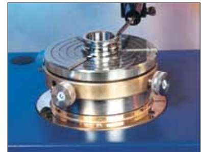
gauge arm in horizontal attitude with orientation downward to measure top face
